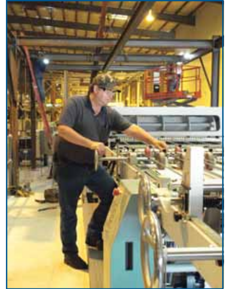
William Bradbury, BOPP Mechanical Supervisor, looks over the new sheeter/cutter equipment currently being installed in BOPP.
