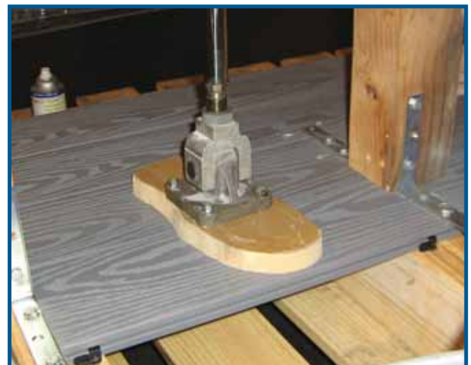
Foot simulator used to demonstrate the durability of TUFdeck®.
